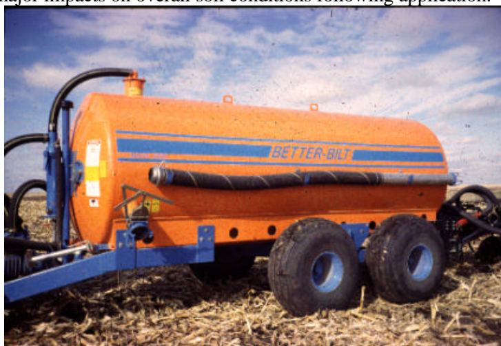
Figure 1. Manure applicator tank.
