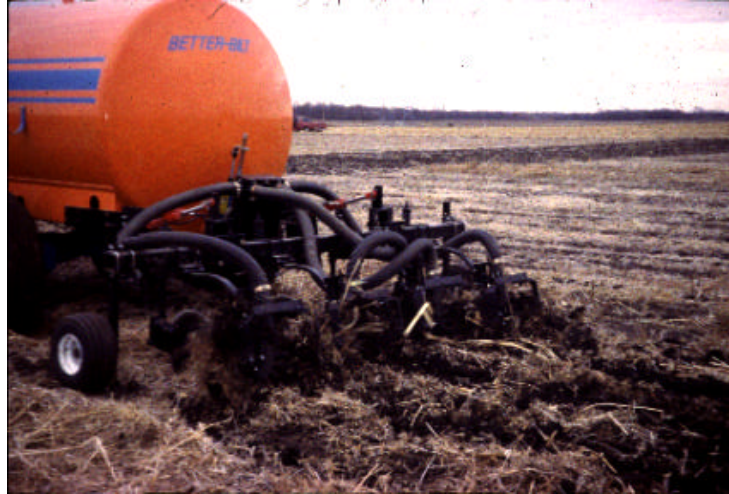
Figure 3. Sweep injectors operated in soybean residue.
