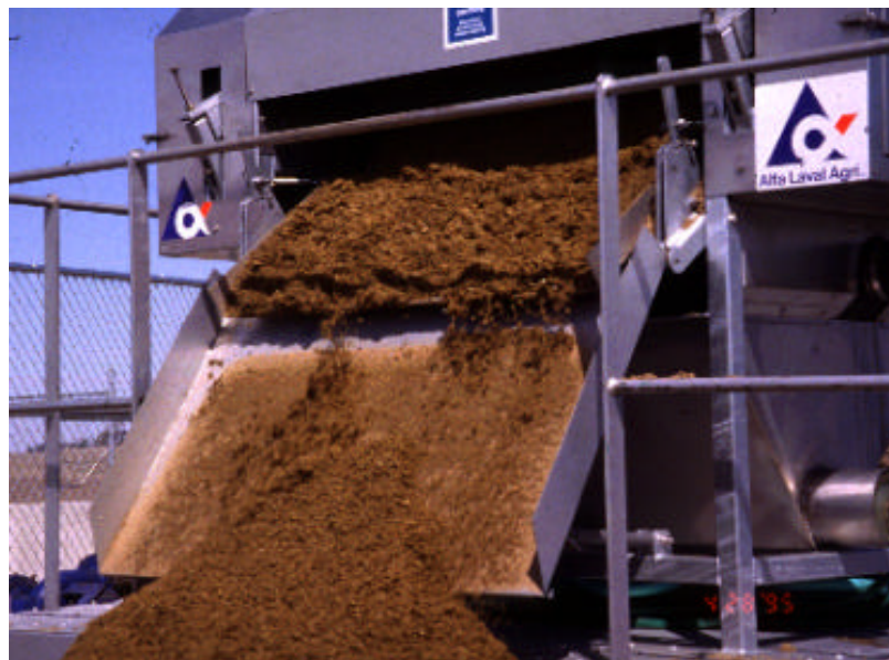
Figure 3. Rotary screen solids separator processing dairy manure
